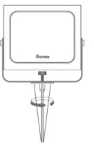
Install each flood light on the ground and adjust the angle of its beam.
